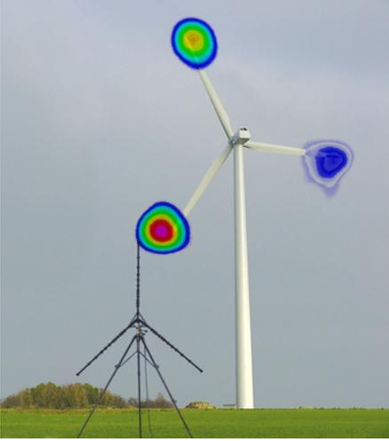
Figure 2: Superimposing of acoustic “heat map” (colormap) and photo for localization of sound sources at a wind turbine (Source: [www.acoustic-camera.com](http://www.acoustic-camera.com))
