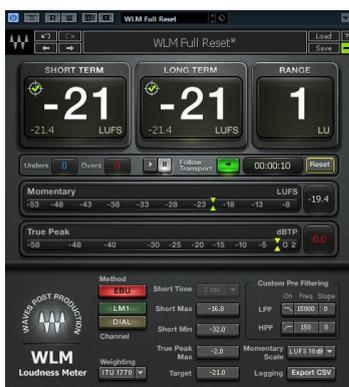
Figure 7. Waves Loudness Meter plugin interface displaying one of the recorded noise LUFS level (Loudness Units Full Scale)
