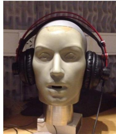
Figure 4. Impulse response measurement using an acoustic dummy head and headphones. The measurement took place in the acoustic laboratory of the UNTREF. Focusrite HP60 were used for the test.
